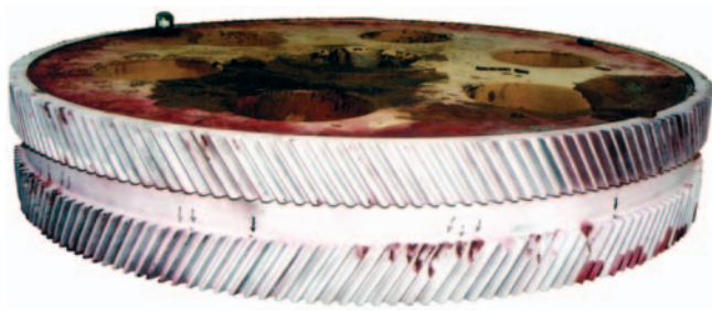
Intermediate Gear / \varnothing 2.2 m, 4 ton
