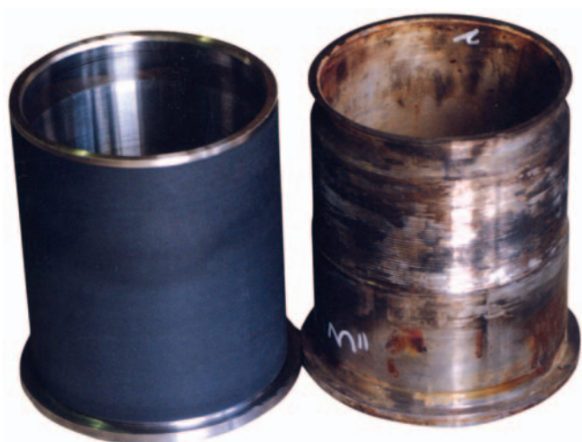
Sleeves Ø240mm: Ceramics increase service life up to 700% than stainless steel.
